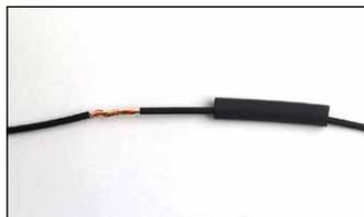
2. Twist wires together and make sure the sleeve is kept away from any heat source
