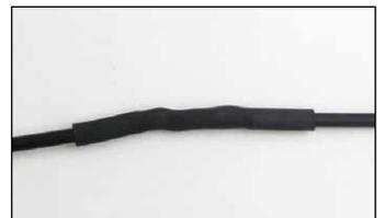
4. Slide the tubing over the connection and apply heat from a heat gun or lighter so it shrinks the sleeve and seals the joint.
