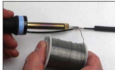
3. Apply heat to the splice from the soldering iron./pen and feed a small diameter, quality 50/50 solder to the iron and let the molten solder absorb into the connection.
