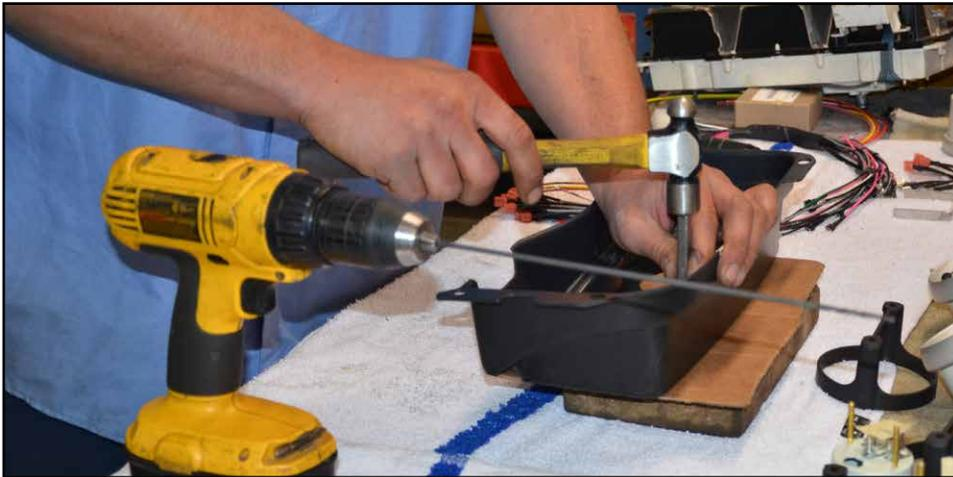
*Prior to drilling the 5/32" holes for the warning lights use a punch and mark where the hole is to be placed. Cement the lights in place.*
